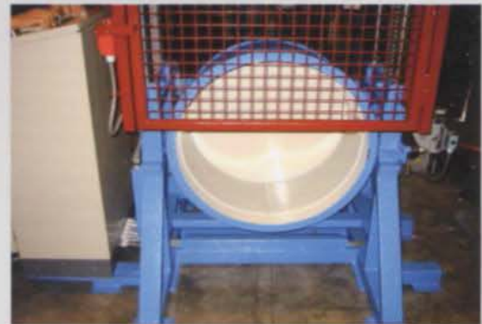
TANK DETAIL DURING THE UNLOADING PHASE PARTICOLARE VASCA IN FASE DI SCARICO DETAIL DE LA CUVE EN PHASE DE VIDANGE
